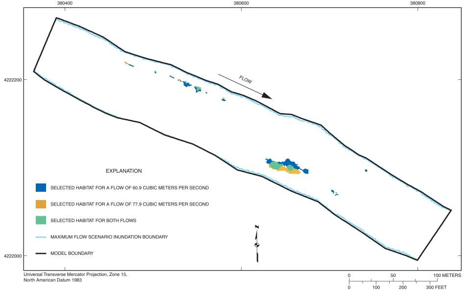
Figure 5-19. Selected habitat area distribution for habitat categories 4, 5 combined (slenderhead darter) at flows of 60.9 and 77.9 cubic meters per second at Marais des Cygnes River site MDC3.
